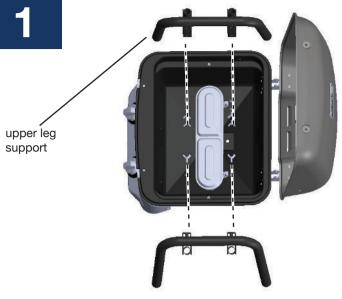
Fit upper leg supports to Barbecue sink using wing nuts and washers provided.
