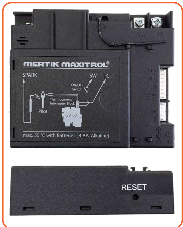
Figure 4.2 | Top and side view of the Receiver
