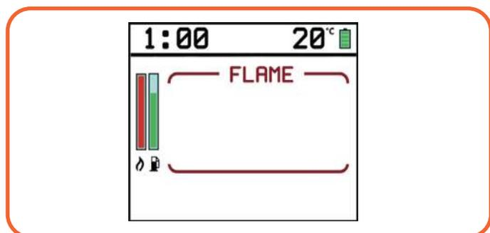
Figure. 4.6 FLAME-mode, burner is turned on
