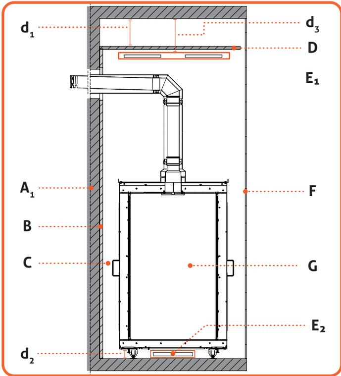
Figure 6.4 | C31: Flue situation Non-Flammable materials
