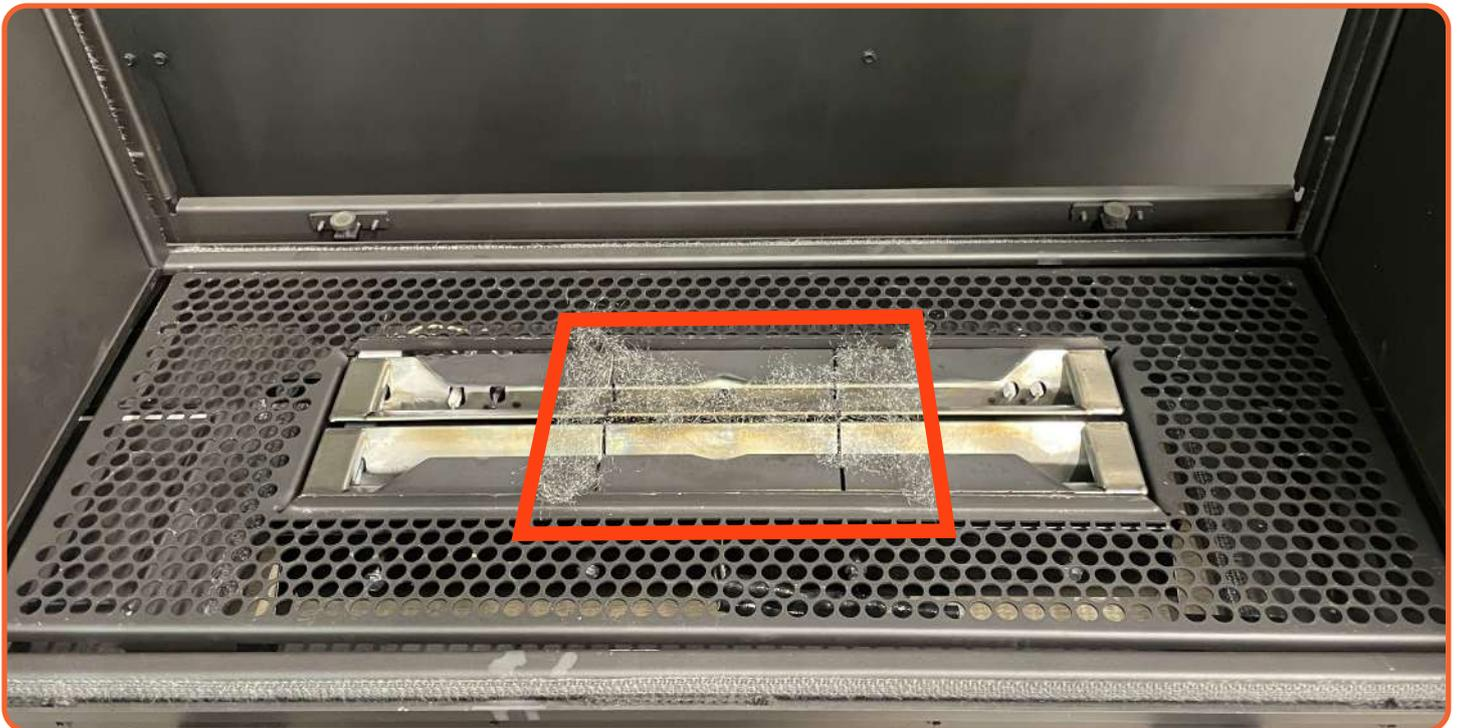
Lay the filament over the burner making sure it is within the orange box remains. The filament must not come into contact with the sensors in the burner.
