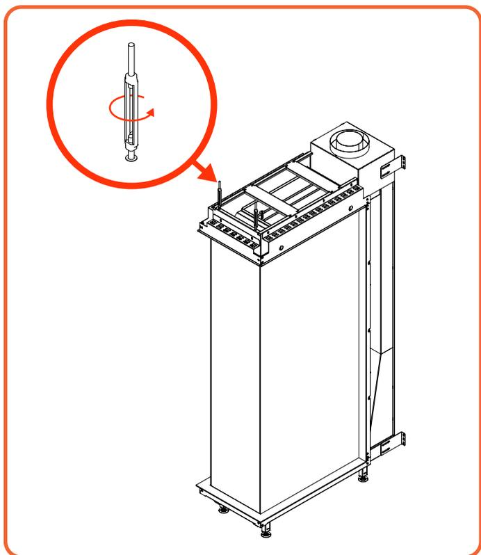
Figure 6.1 | Turnbuckles to mount fire to ceiling
