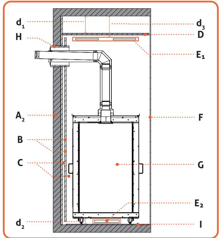
Figure 6.2 | C31: Flue situation Flammable materials
