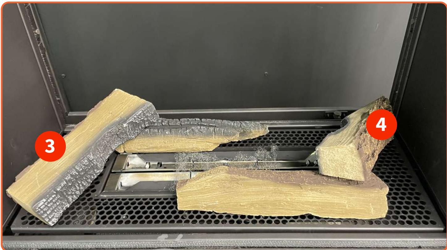
Place logs 3 and 4 with the hole at the bottom on the pin of the underlying log.
