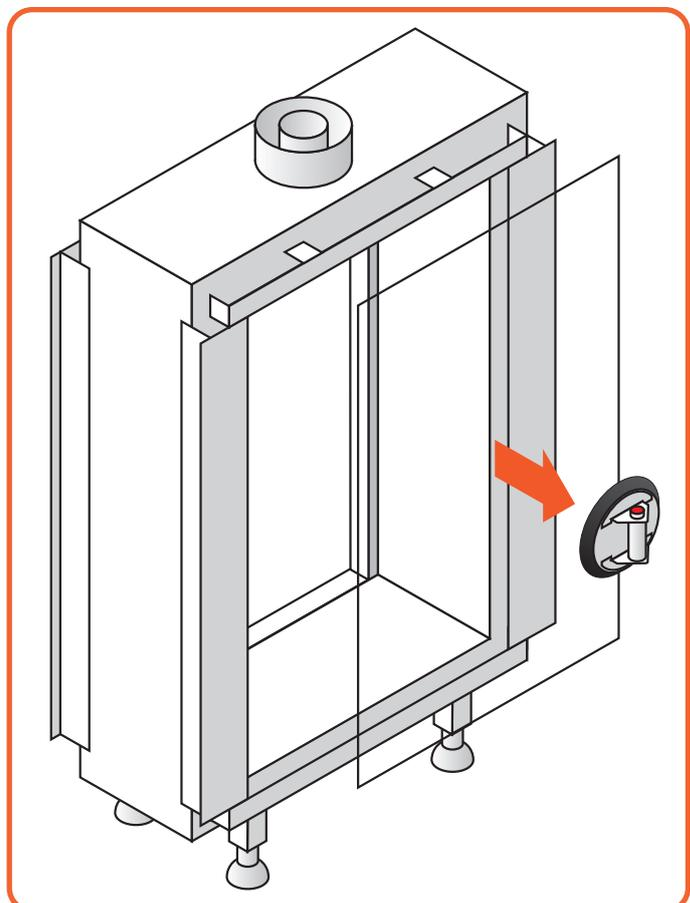
Figure 10.9 | Carefully lift the glass out of the fireplace
