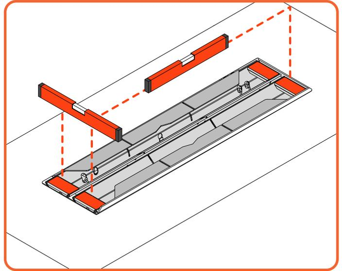
Figure 5.3 | Make sure the burner is level
