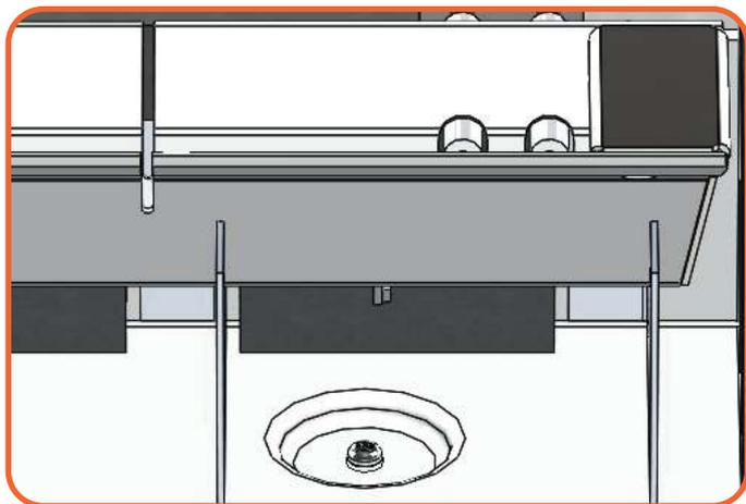
Figure 8.1 | Leak detection sensor underneath burner
