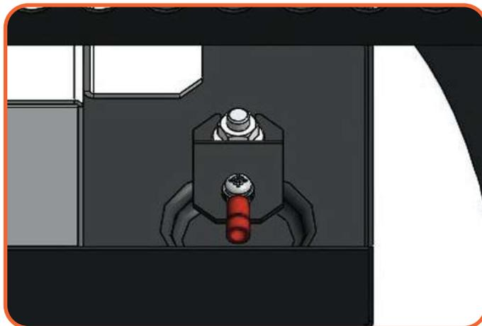
Figure 8.2 | Leak detection sensor on lowest point
