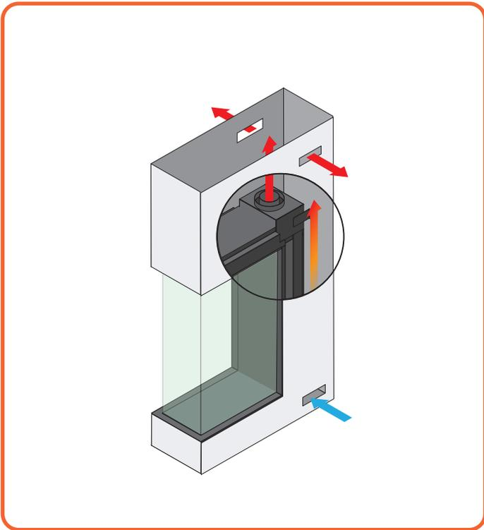
Figure 5.1 | Flueless installation
