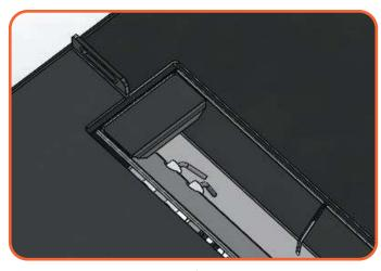
Figure 8.3 | Overflow detection sensor
