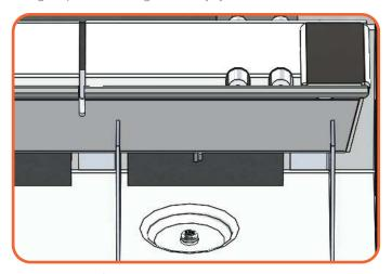
Figure 8.1 | Leak detection sensor underneath burner
