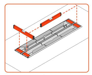
Figure 5.3 | Make sure the burner is level
