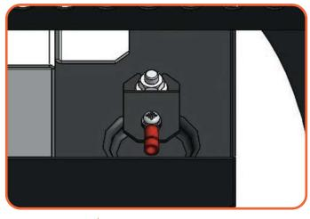
Figure 8.2 | Leak detection sensor on lowest point
