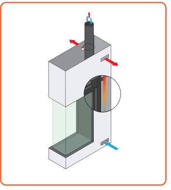
Figure 5.2 Balanced flue installation
