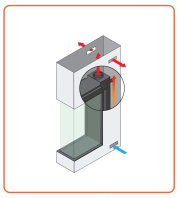
Figure 5.1 | Flueless installation
