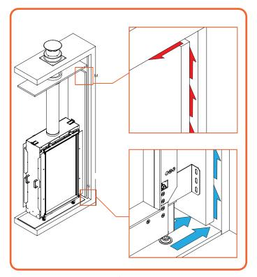
Figure 6.6 | Air flow between wall covers
