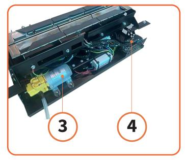
Figure 11.2 | Fillpump en fuel pump
