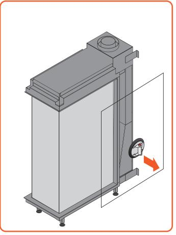
Figure 9.7 | Carefully lift the glas out of the fireplace
