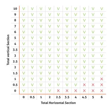
Attention: For fireplaces is this flue category it is possible to reduce the flue from a size 200/130 to a 150/100 flue, when the flue is exclusively vertical.
